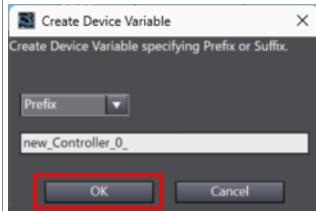
The HMI-side device variables are generated.
