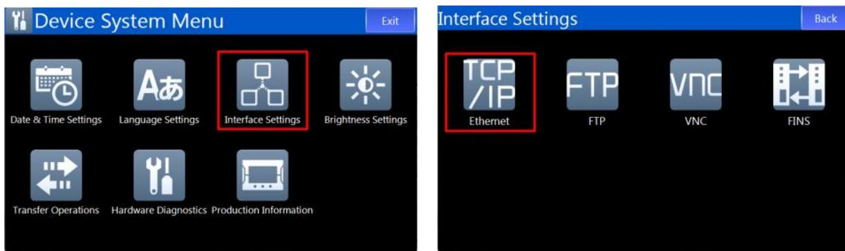
Enter the IP address and subnet mask in the Ethernet settings and press the [Apply] button.
