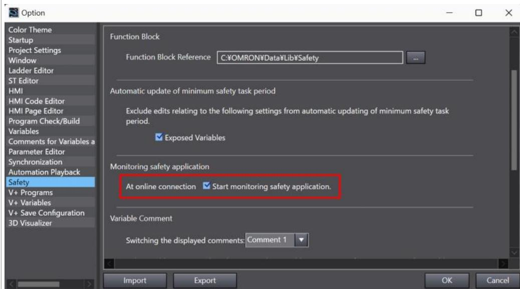
You can start monitoring the safety application by selecting the icon button shown in the red frame in the figure below in the safety project.
