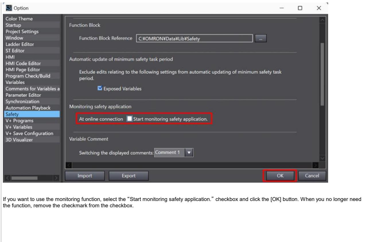
If you want to use the monitoring function, select the “Start monitoring safety application.” checkbox and click the [OK] button. When you no longer need the function, remove the checkmark from the checkbox.
